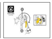
The AUTO-LOCK system allows users to easily position themselves at a work station without having to manipulate the handle or tie off the device: as soon as the user releases the handle, the rope is automatically locked in the device.
