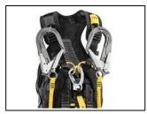
The MGO connectors on ABSORBICA fall arrest lanyards can be stowed on each shoulder strap. The user is thus unhindered by the lanyard, and the connectors stay within reach. In case of a fall, a system releases the MGO connectors to allow the absorber to be deployed.
